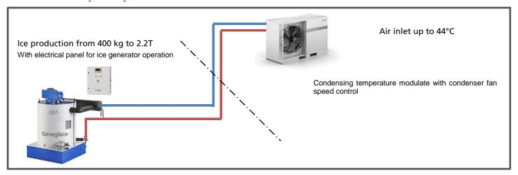
GEA GENEGLACE makes also available a simple "quick selection curve" that will help you to make the right material selection considering the external conditions and the desire ice production. The SPLITPACK will be sold as a complete set of production excluding refrigerant and local connections.
